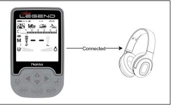
Power off the detector and the headphones. Then, power the headphones back on. The green LED on the headphones will start blinking.
